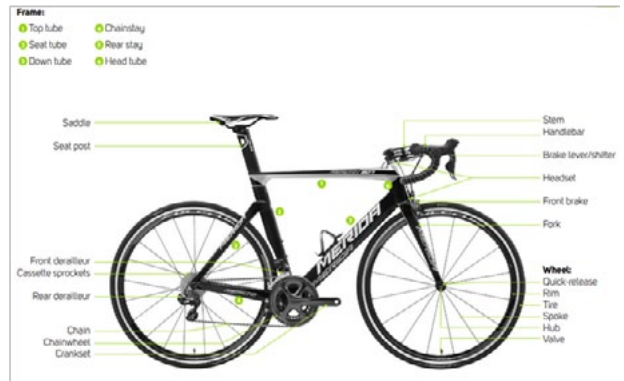
Figure 4 Components of a bike, Courtesy: Merida and TBA.
